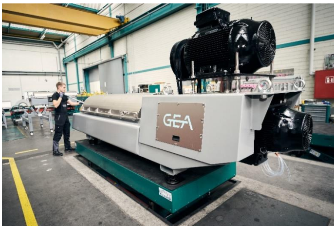
Figure 2: GEA has been producing decanter centrifuges at the Niederahr site for over 60 years. These are deployed, for example, in water treatment, lithium processing, protein extraction as well as the beverage and dairy industries. (Photo: GEA/Marcel Häbel)
